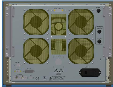
**Figure 2-2. Model 500A250D Rear Panel**
