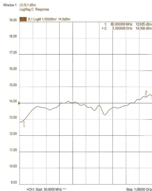
Figure 4-8. Typical A2 Driver Module Response
