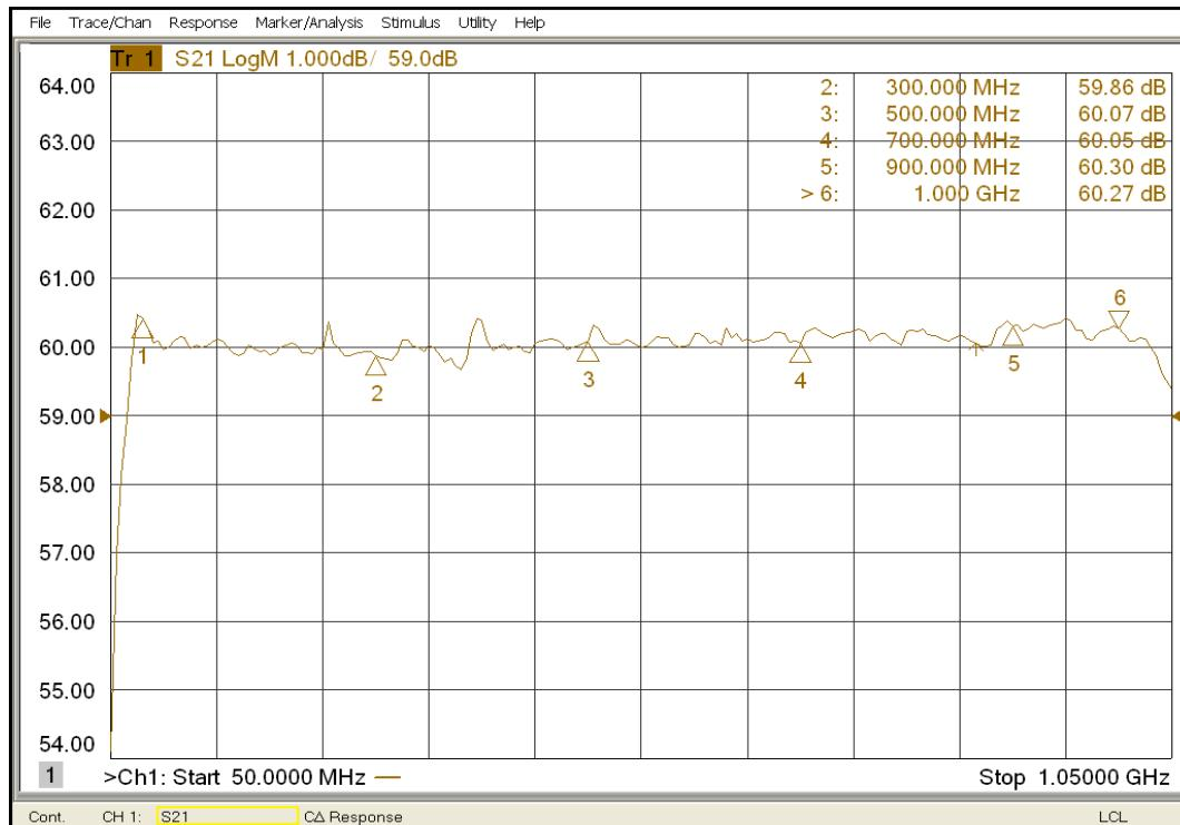
Figure 4-1. Typical Response at 0 dBm Input
