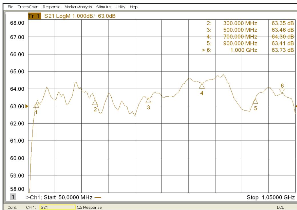
**Figure 4-2. Typical Response at -20 dBm Input**
