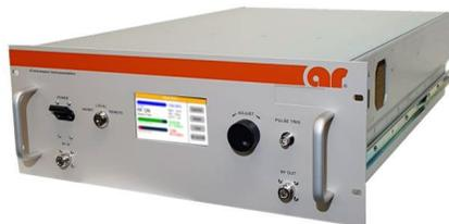
The Model 1500/1000SP1z2G3z1 is equipped with a Digital Control Panel (DCP) which provides both local and remote control of the amplifier. The DCP uses a color LCD touch screen and a single rotary knob to offer status reporting and control capability. The display provides Forward Power and Reflected Power values plus amplifier status. Special features include a gain control and RF output level protection.
