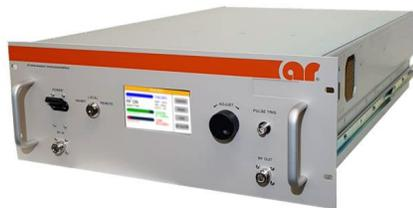
The Model 2000SP1G2 is equipped with a Digital Control Panel (DCP) which provides both local and remote control of the amplifier. The DCP uses a color LCD touch screen and a single rotary knob to offer status reporting and control capability. The display provides Forward Power and Reflected Power values plus amplifier status. Special features include a gain control and RF output level protection.
