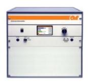
The Model 250\$1\$G6 is a solid-state, Class A design, self-contained, aircooled, broadband power amplifier designed for applications where instantaneous bandwidth, high gain and linearity are required. It will provide a minimum of 250 W across its operating bandwidth. Protection from input overdrive beyond 0 dBm is provided as well as protection from various failure conditions including over-temperature and power supply faults.
