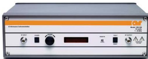
The 30S1G6, when used with a sweep generator, will provide a minimum of 30 watts of RF power. Included is a front panel gain control which permits the operator to conveniently set the desired output level. The 30S1G6 is protected from RF input overdrive by an RF input leveling circuit which controls the RF input level to the RF amplifier first stage when the RF input level is increased above 0 dBm. The RF ampli-
