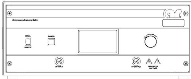
Figure 2-1. Model 40S6G18-L Front Panel
