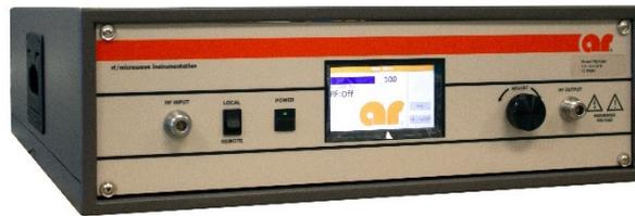
The Model 75S1G6C is a solid-state, Class A design, self-contained, air-cooled, broadband power amplifier designed for applications where instantaneous bandwidth, high gain and linearity are required. It will provide a minimum of 75 W across its operating bandwidth. Protection from input overdrive beyond 0 dBm is provided as well as protection from various failure conditions including over-temperature and power supply faults.
