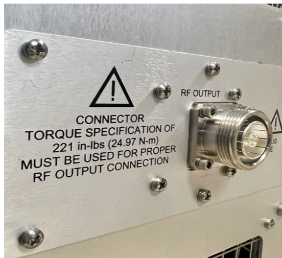
Figure 2-3. Rear Panel 7-16 DIN Connector
