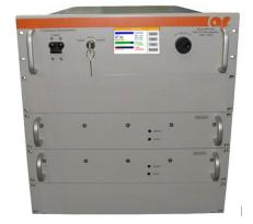
The Model 4000SP0z8G2z5 is equipped with a Digital Control Panel (DCP) which provides both local and remote control of the amplifier. The DCP uses a color LCD touch screen and a single rotary knob to offer status reporting and control capability. The display provides Forward Power and Reflected Power values plus amplifier status. Special features include a gain control and RF output level protection.
