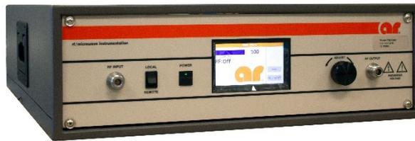
The Model 125W1000A is a solid-state, Class A design, self-contained, air-cooled, broadband power amplifier designed for applications where instantaneous bandwidth, high gain and linearity are required. It will provide a minimum of 125 W across its operating bandwidth. Protection from input overdrive beyond 0 dBm is provided as well as protection from various failure conditions including over-temperature and power supply faults.
