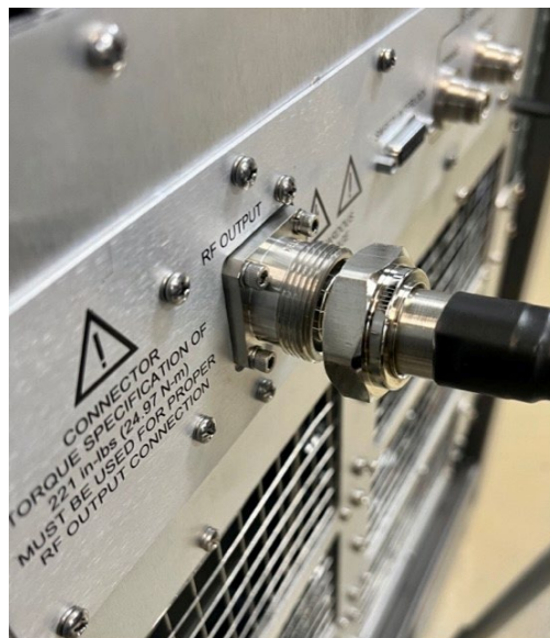
Figure 2-4. Align Connectors for Interface
