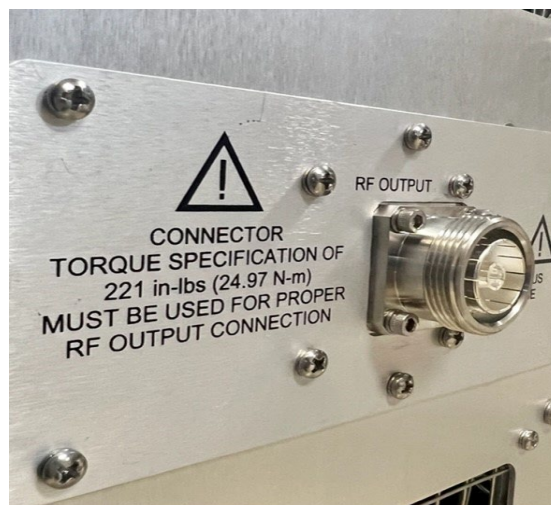
Figure 2-3. Rear Panel 7-16 DIN Connector
