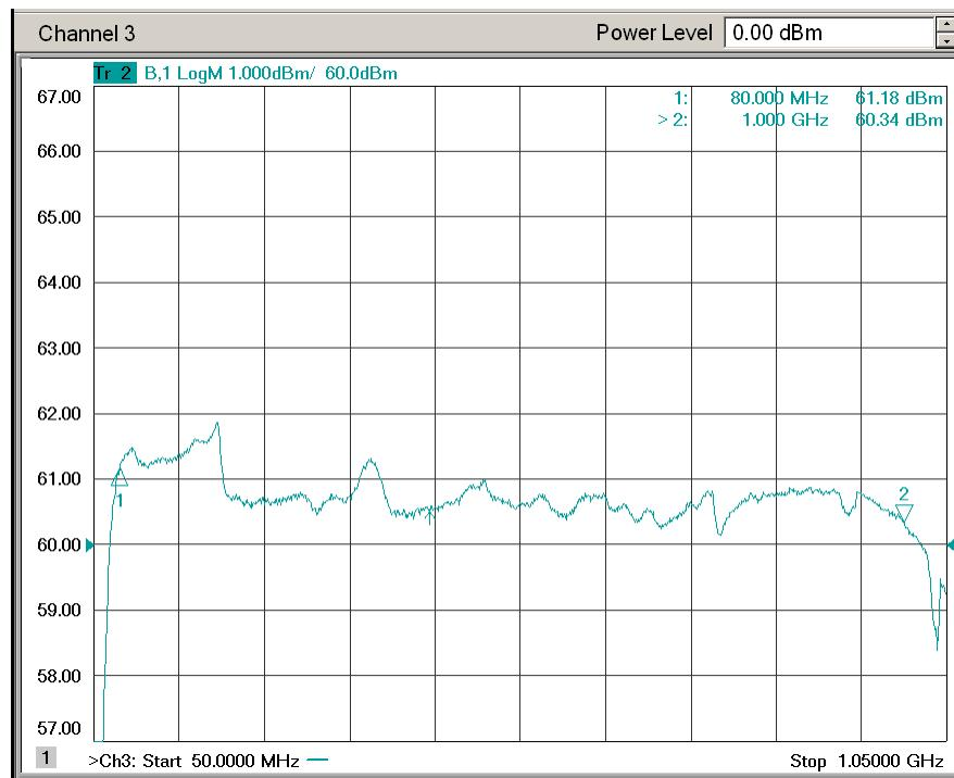
Figure 4-2. Typical Response at 0 dBm Input
