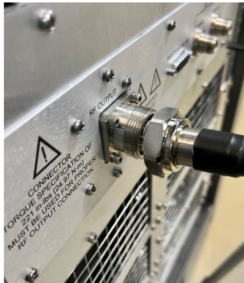
Figure 2-4. Align Connectors for Interface
